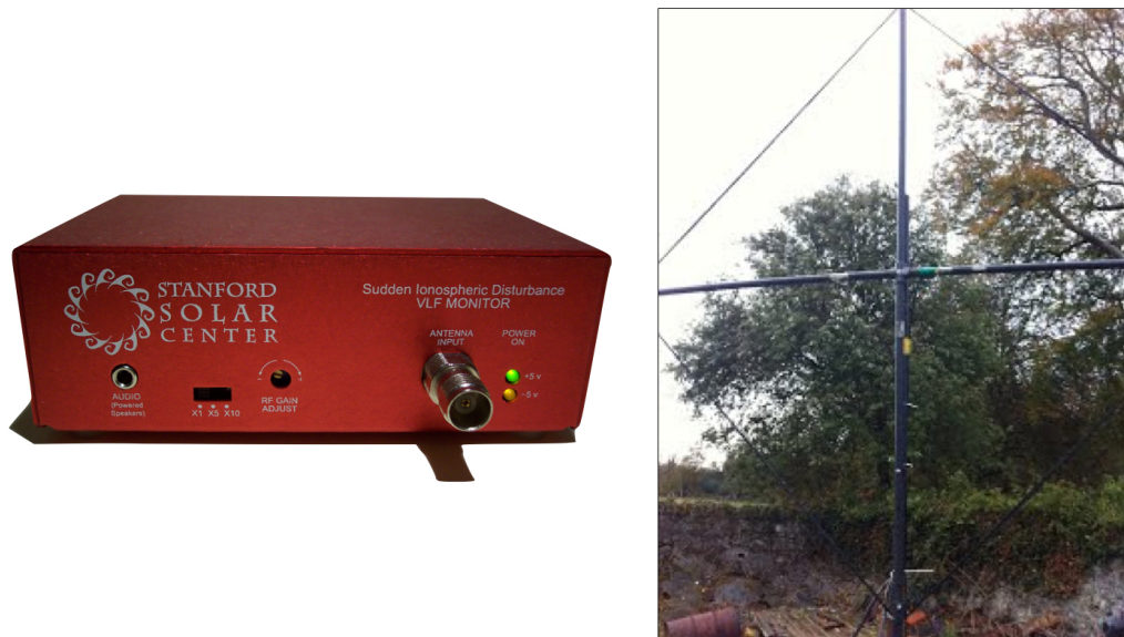
Figure 3.9: The Stanford SID monitor (left) and the wire-loop antenna (right) that make up the VLF receiving system. This system is located at the Rosse Solar Terrestrial Observatory in Birr, Co. Offaly Ireland and receives VLF signals at 24 kHz.
