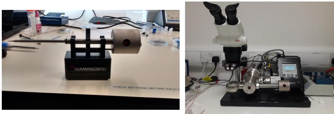
Figure 4.2: The liquid cell holder and the pumping station. Cells are assembled, and the integrity of the assembled cell is verified using the high vacuum chamber in the pumping station.
