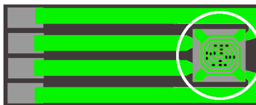
Figure 2.6 Schematic of standard in-situ TEM sample heating chip. White circle indicates magnified region. Image is not to scale. Adapted from DENS Solutions Inc..
