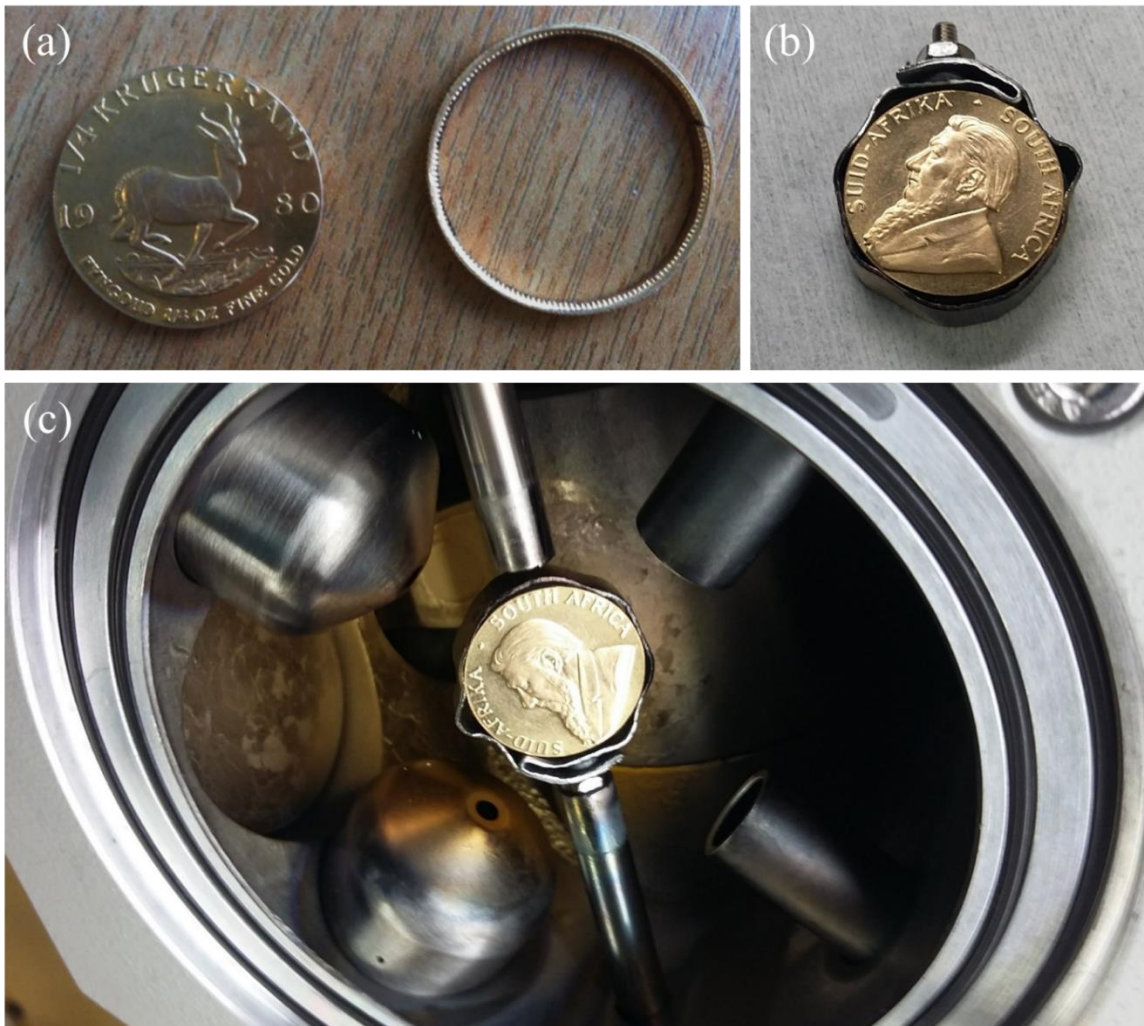
Figure 6.4: preparation of Krugerrand coin for film deposition. (a) Krugerrand after reducing the radius to the correct size, (b) the Krugerrand in the sputtering target holder, (c) the Krugerrand in the deposition chamber of the sputtering system.
