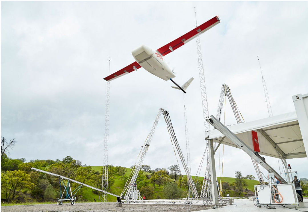
Figure 6.2: A fixed-wing UAV launched from a catapult. Image used with permission from : [124]
