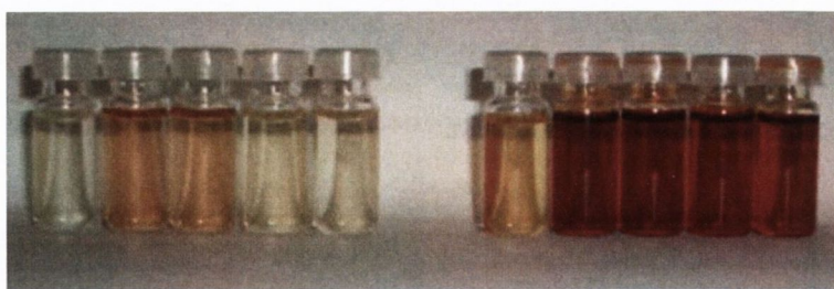
Figure 1.14 DMSO solutions ( 2 \times 10^{-3} M) of 40 (left set) and 42 (right set). From left to right in each group: solution of receptor, followed by solutions with receptor in the presence of 1 equiv. of fluoride, acetate, benzoate and dihydrogenphosphate. 88
