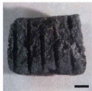
Figure 4.40. Comparative MTT staining of surface and longitudinal cross-sections of bimodal and trimodal scaffolds 5 days post seeding. Scaffolds were subjected to either static or dynamic culturing. Scale bar is 1mm.
