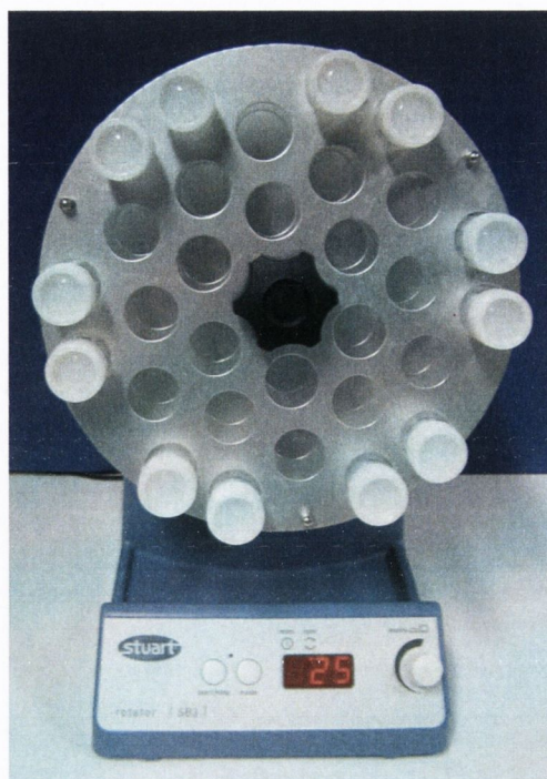
Figure 3.29. Experimental setup for dynamic rotational seeding of HA scaffolds.
