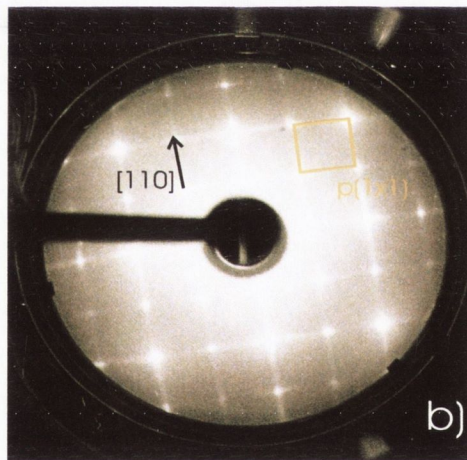
Figure 6.6: a) AES spectrum of low-level contaminated surface. 1.3 % of Ca has been found at the surface of the crystal. b) LEED pattern, taken with a primary electron energy of 90 eV, corresponding to a p(1 \times 1) streaked superlattice, marked with a yellow square.
