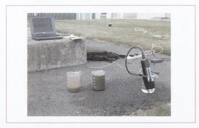
Figure 8. 7 Photograph showing the use of the SCUFA to indicate the tracer concentration
