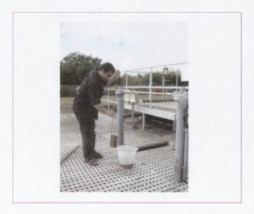
Figure 8. 10 Photograph showing the sampling of the effluent
