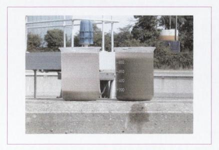
Figure 8. 6 Photograph showing the settlement of the bacteria flocs to reveal the clear supernatant
