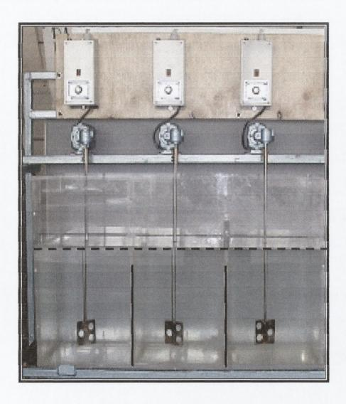
Figure 6. 9 Photograph showing three CSTR in-series model
