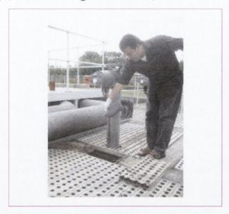
Figure 8. 9 Photograph showing the injection of the tracer into the system
