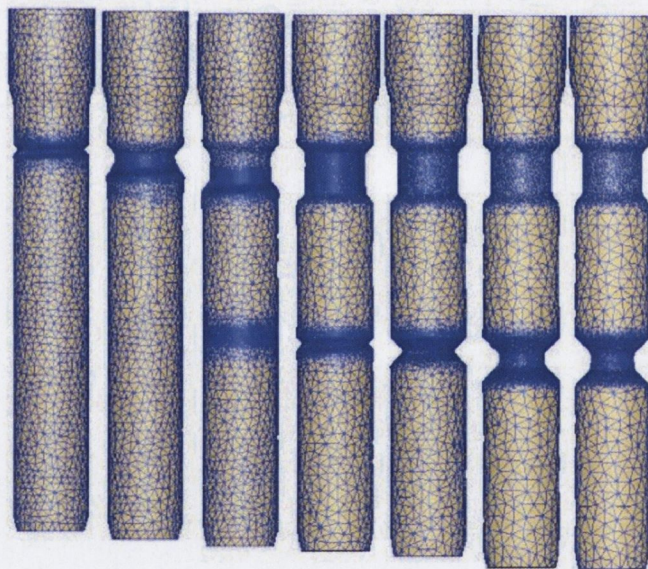
Figure 5.2 FEA representation of the progression of Form Rolling a Double Groove feature onto a workpiece shown for every 360° rotation.
