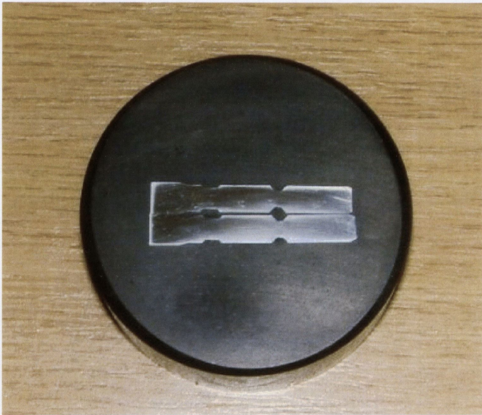
Figure 4.8 Mounted longitudinal sections of a complete Double Groove workpiece.
