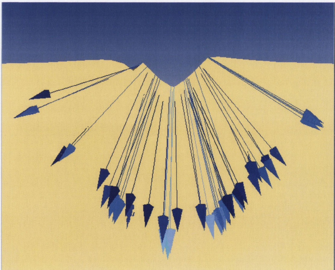
Figure 5.16 Vector plot of material flow for a cross-section taken through the first groove after 180° fastener rotation.
