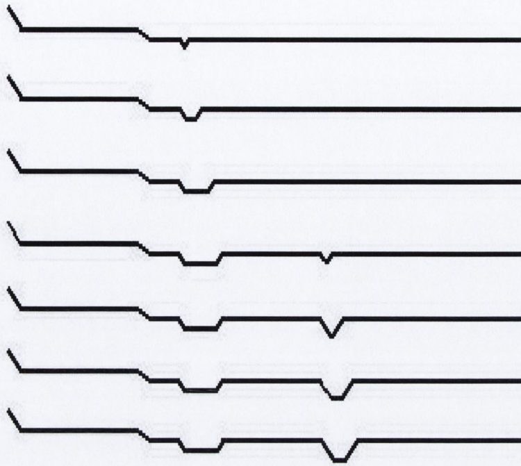
Figure 4.5 Fastener cross-sections during Form Rolling in increments of 360^\circ rotation.
