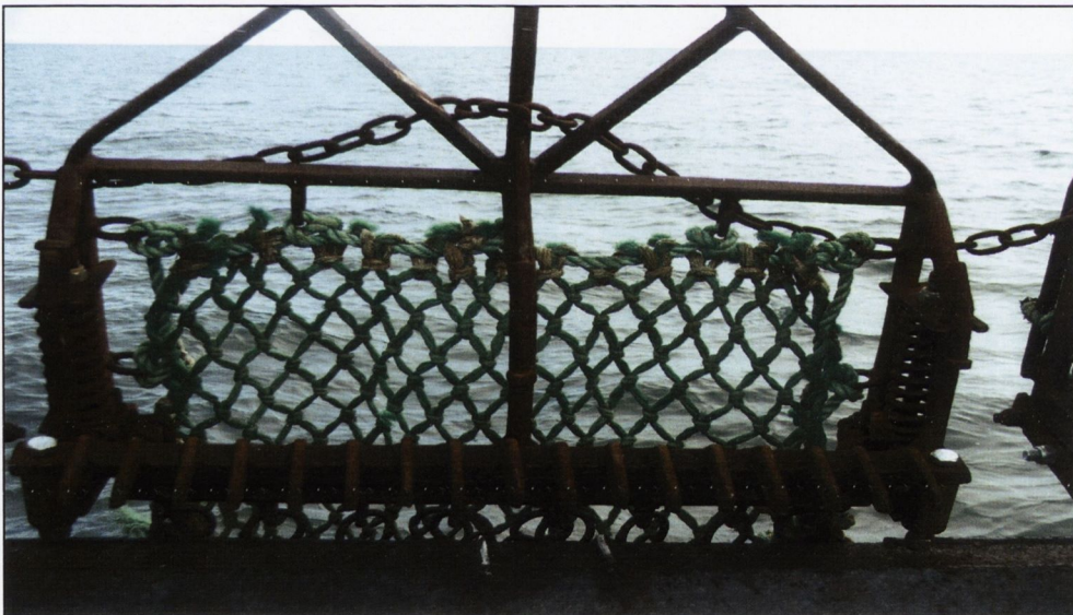
Figure 5.1 Scallop dredge used during the scallop survey. Above, view of six dredges on tow bar. Below, close view of dredge frame.
