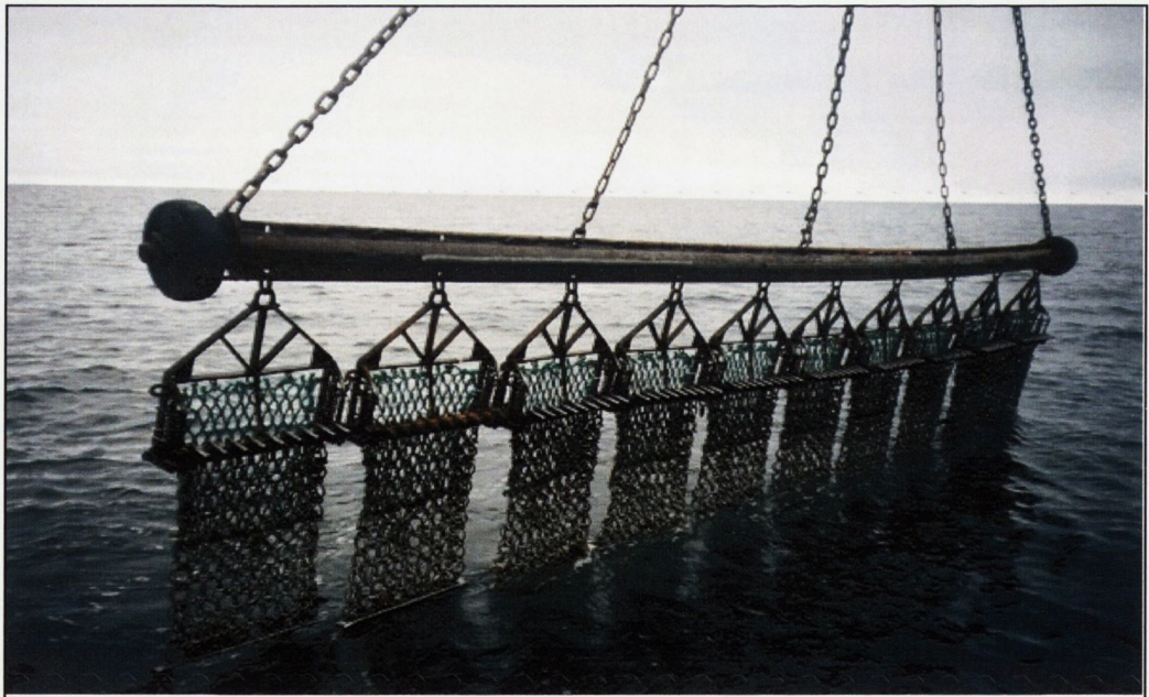
Figure 1.10. Commercial spring loaded scallop dredges suspended on a beam being deployed from a commercial fishing vessel.
