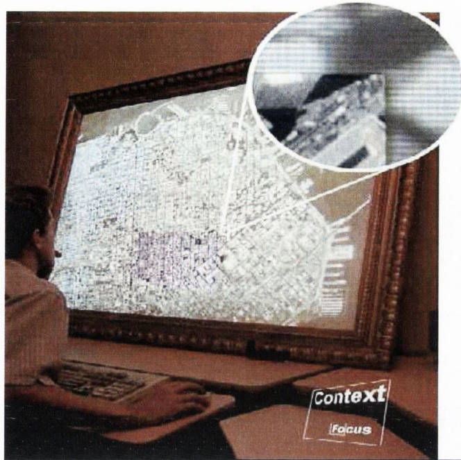
Figure 2.3: A Focus Plus Context Screen. (Image from [BDDG03] courtesy of Andrew T. Duchowski.)
