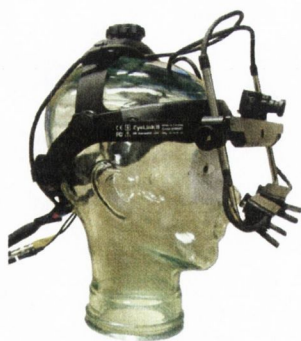
Figure 2.2: EyeLink II eye-tracker with scene camera.
