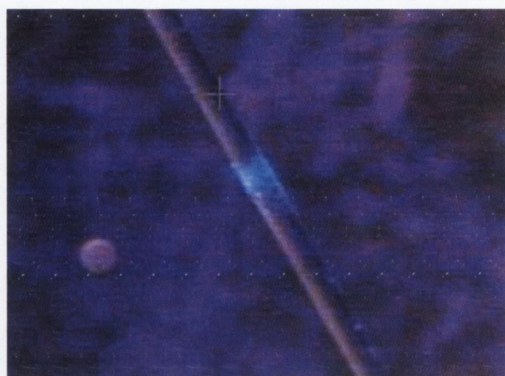
Figure 6-28 Microscope image of 80 \mu\text{m} ring formed on surfacesilane- treated fiber.
