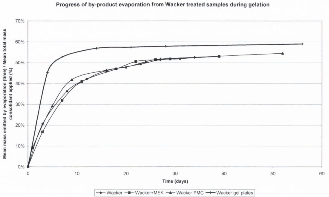
Figure 6.14: Progress of by-product evaporation from Wacker treated samples and gels during condensation
