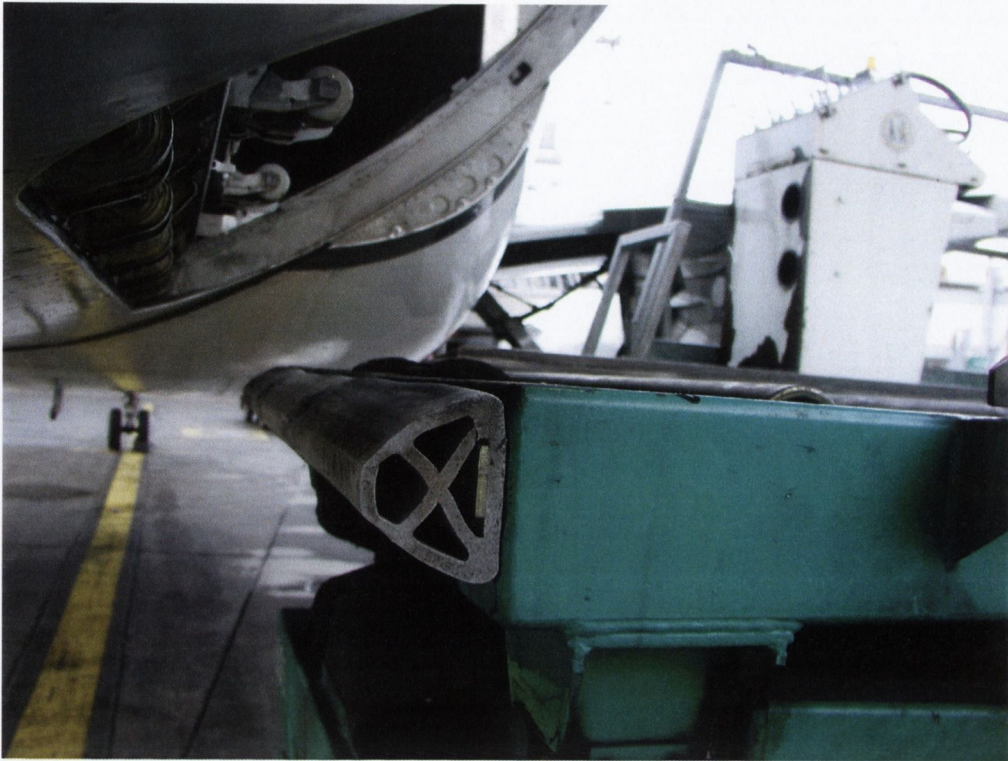
Figure 2.7 Rubber pads to safeguard against impact
