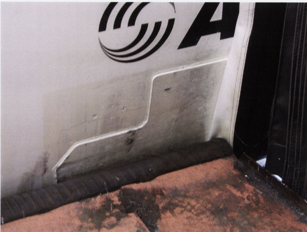
Figure 2.8 Repair of impact damage to front entry door of Airbus A320 at Dublin Airport
