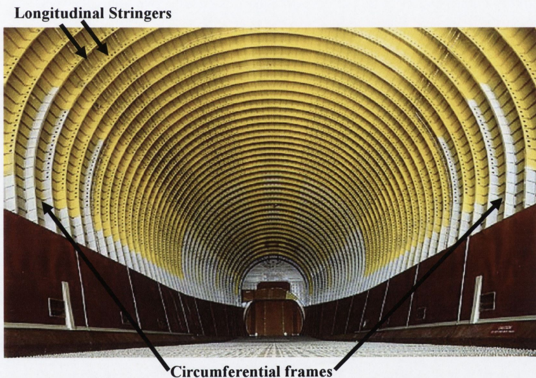
Figure 2.1 Beluga fuselage, internal view showing semi-monocoque design
