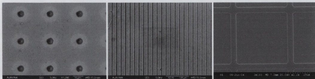
Figure 12: Silicon oxide substrates patterned by soft lithography. Catalyst particles are present within the patterns (darker regions) and absent elsewhere.
