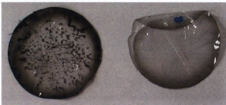
Figure 4.4 – Photograph of MWNT/First Contact films dried in petri dishes. The darker regions at the edges are due to drying effects, which cause a higher MWNT concentration at the edges. The films shown are ~49 mm in diameter.
