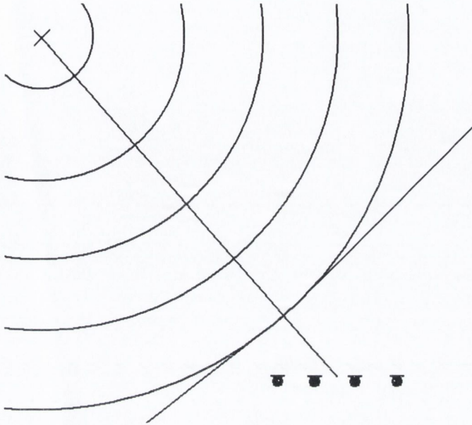
Figure 5.3: The far-field assumption: For distant sound sources, the curvature of the incident wavefront is negligible.
