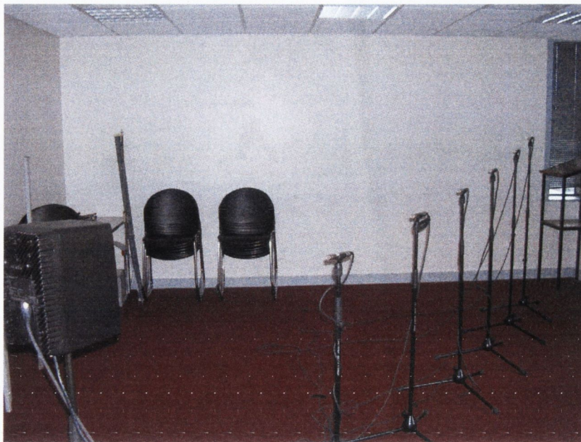
Figure 2.7: A photograph of the experimental setup used to obtain DRRs at varying distances from a sound source.
