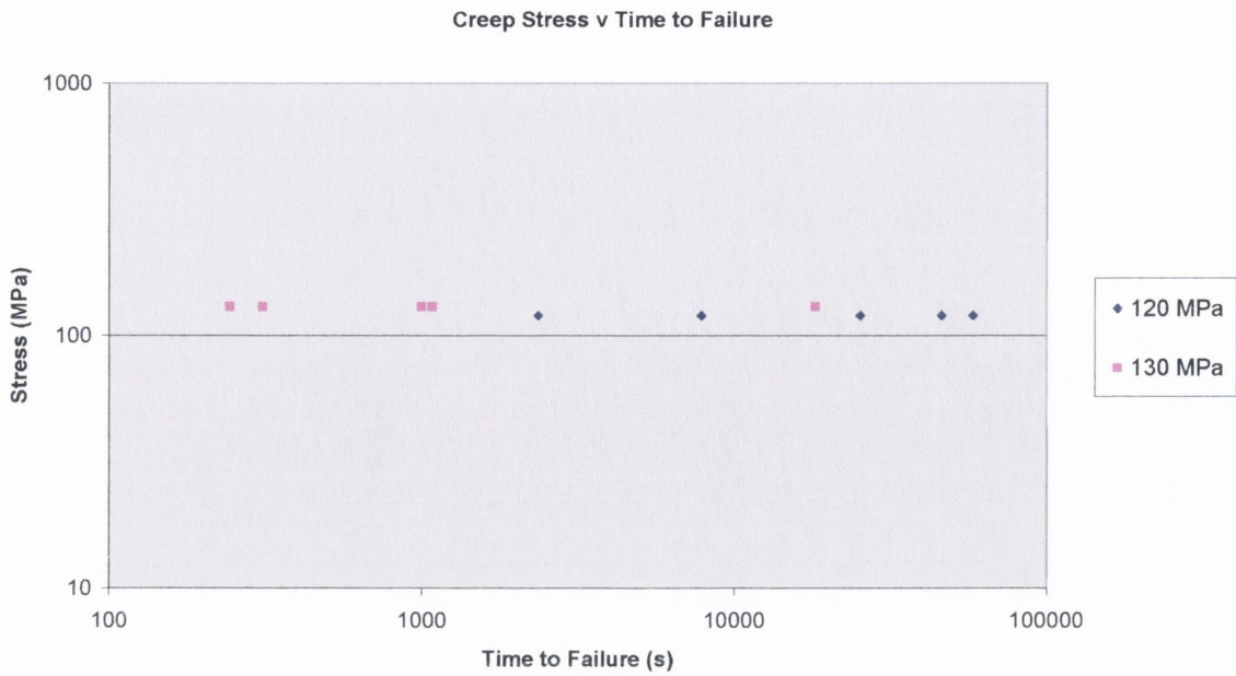
Fig. 3.56 Log-log plot of stress versus time to failure for all high temperature creep specimens
