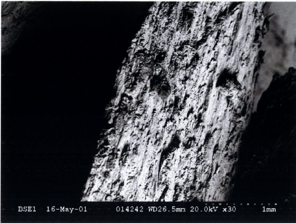
Fig. 3.34 Scanning electron micrograph of the fracture surface of a specimen tested at 140 MPa, x30 magnification (appendix 2.1 specimen 17)
