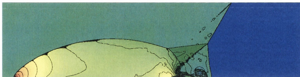
Figure 3-5: Isopycnics for double Mach reflection, parameters are \alpha=60^\circ , \gamma=1.4 , M=10 . This compares well with published results using this test (Woodward & Colella 1984; Stone & Norman 1992; Berger & Colella 1989). Main features visible include the contact discontinuity roll-up along the lower right of the image, launching a jet of dense material towards the Mach stem and causing it to bulge outwards, the triple point or lambda point where the three shocks meet and the wall heating error where the perfect resolution at the a priori boundary condition contrasts with the slight smearing by the numerical code.
