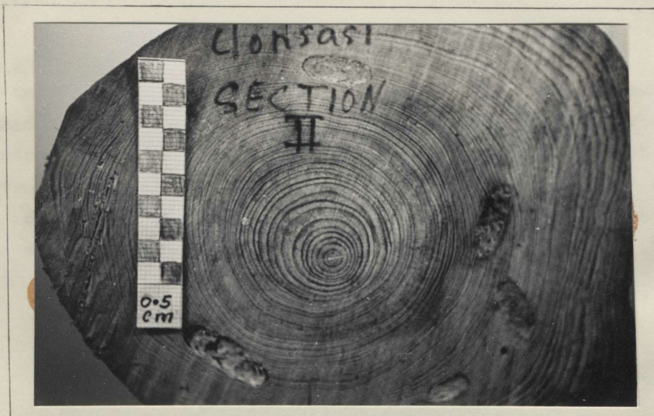
Photograph of Section II in which holes due to borers are visible.
