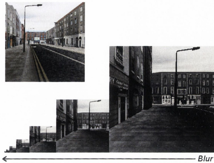
Figure 5.7: Gaussian pyramid for an input image (top left) based on the intensity channel of the image. Each level is successively filtered and decimated (from right towards left).
