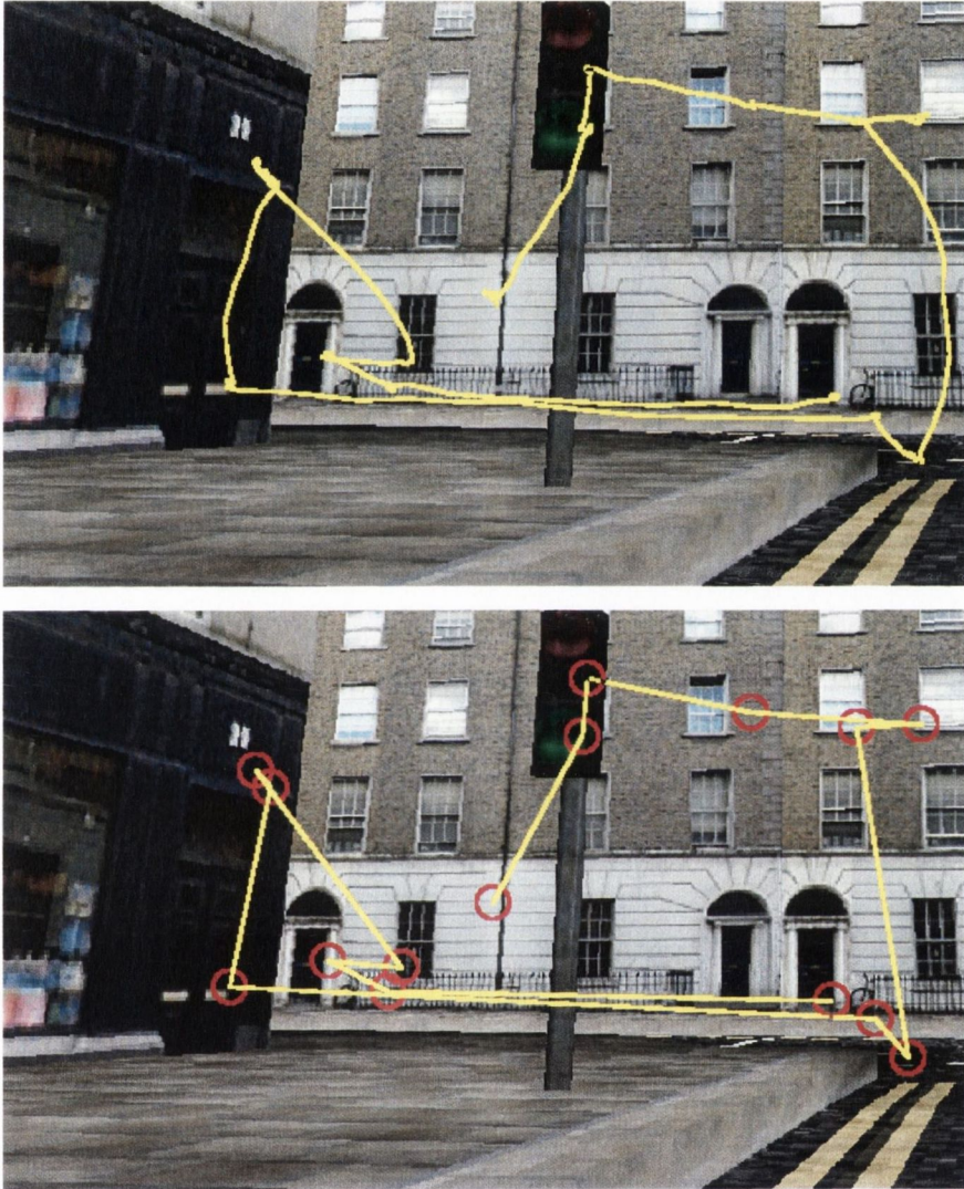
Figure 6.9: Human fixations and scanpaths from a scene in a virtual environment captured using eye tracking equipment. The raw eye data (top image) is processed into saccades, denoted by yellow lines, and fixations, denoted by red circles (bottom image). It is the task of the attention system to provide analogous data to the gaze generation module based on the visual input from the scene.
