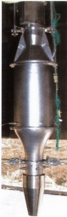
FIGURE 4.4: Close-up of the JEAN nozzle
