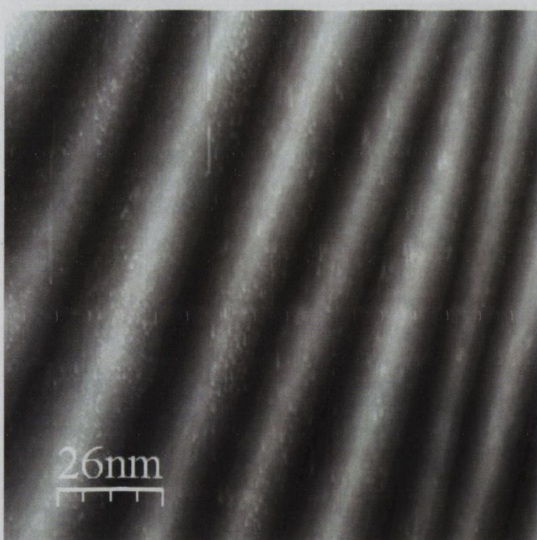
Fig. 8.7: STM after annealing the sample in oxygen at 250 °C at 1 \times 10^{-6} Torr for one hour.
