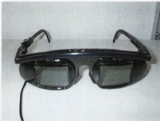
Figure 3.5: 3D Stereoscopic Shutter-Mechanism Glasses.
