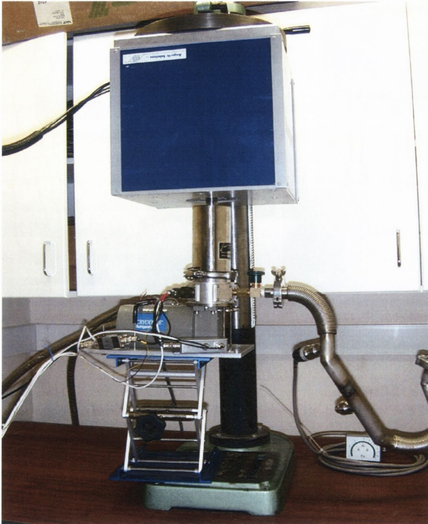
Figure 3.35. Photograph of the CCR 2 system in MR measurement configuration. The measurement head is inserted into the permanent magnet.
