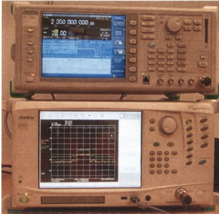
Fig. 8.1: Vector signal generator and signal analyser used for experimentation.
