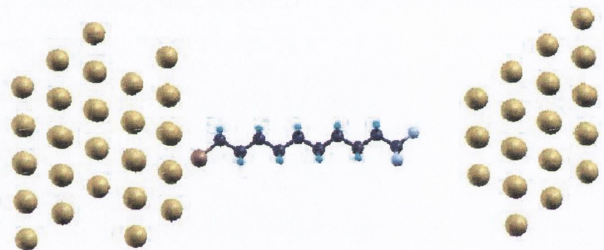
Figure 7.7: Decanethiol molecule attached to gold surface with STM tip with \text{CF}_3 -endgroup. Colour code: Au=yellow, C=black, S=brown, H=blue, F=purple.
