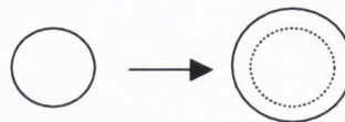
(b) Hydrostatic stress. Causes a change in cell volume, but no change in shape.
