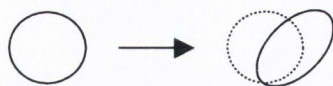
(a) Octahedral shear stress. Causes a change in cell shape, but no change in volume.
