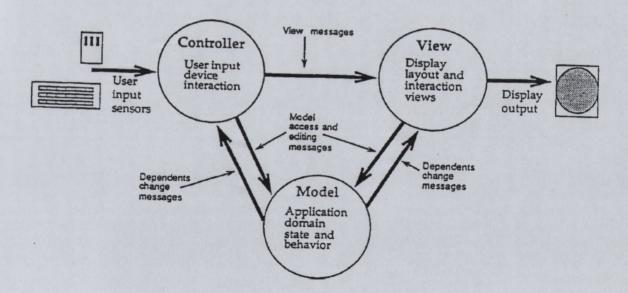
Figure 2.1: The Model-View-Controller pattern (reproduced from [66])
