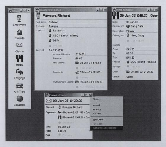
Figure 5.1. An early-stage prototype for an expenses processing system using the Naked Objects framework.
