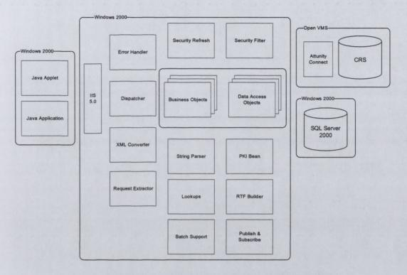
Figure 4-4 Logical architecture of the Naked Object Architecture
