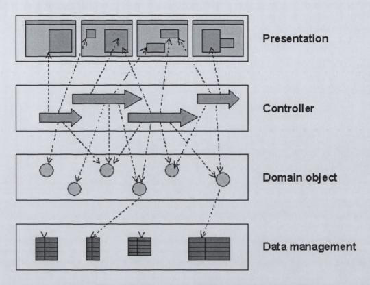
Figure 2.2: The architectural pattern adopted by most business systems is based on four generic layers.
