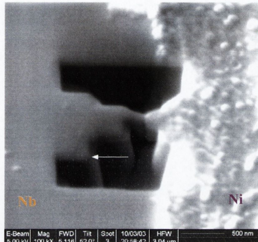
Figure 3.25. The white arrow marks the boundary between Nb and SiO 2 . The picture shows a reduction of the thickness of the Nb film at the constriction due to a bad focussing of the ions.
