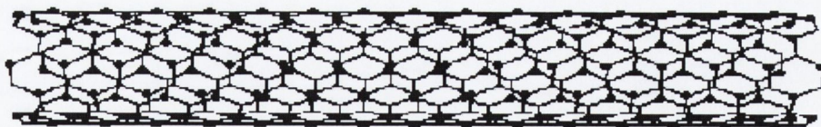
Figure 2.11 Section of a singlewalled carbon nanotube
