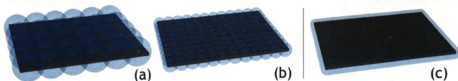
Figure 4.1: Bounding volume fitting for a flat rectangular shape
