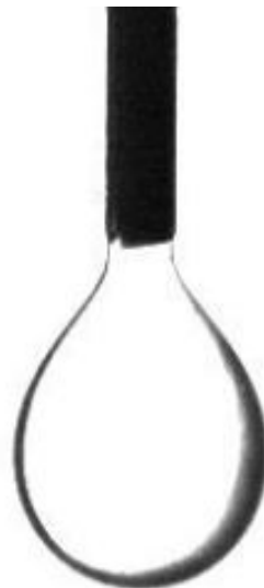
Figure 4.7: Example of a pendant drop. Image credit: Steven Burke, TCD Foams group.
