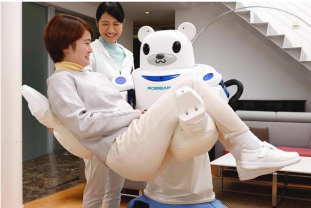
Figure 2-2: Robear lifting a human [30].
