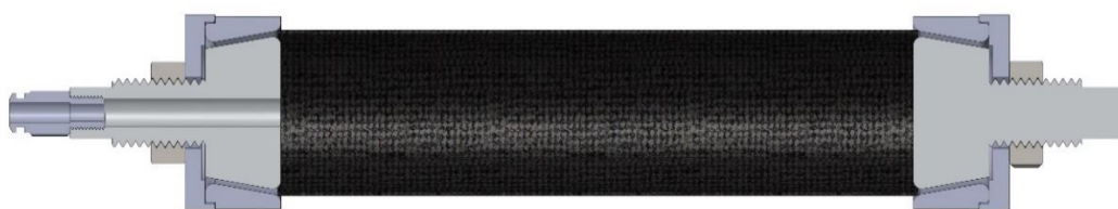
Figure 3-18: Cross section of the standard McKibben muscle.
