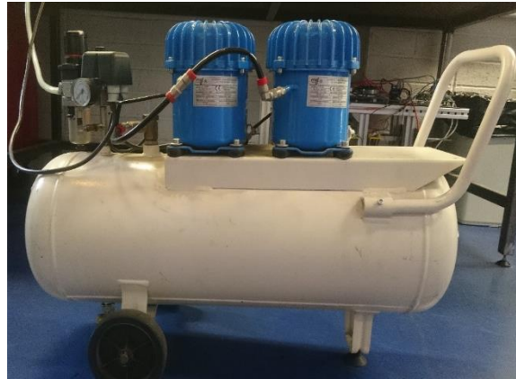
Figure 5-3: The MGF SIL-EOI 50/100 air compressor used in the testing apparatus, with the AWG30-F02G1H filter and manual pressure regulator attached.
