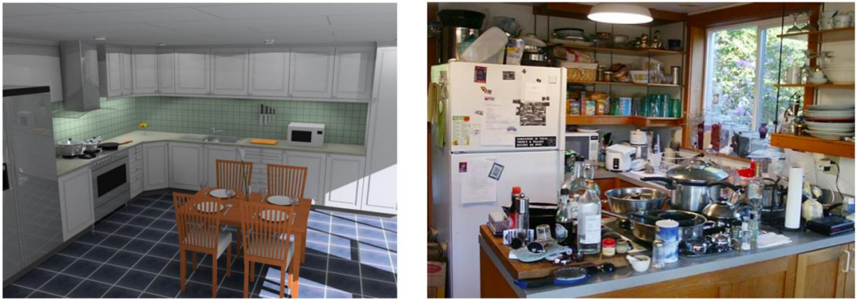
Figure 2-6: An idealised kitchen environment (left) where traditional model-based approaches to robot manipulation and safety are appropriate and the alternative real-world environment (right) where perception and model building is more difficult [55].
