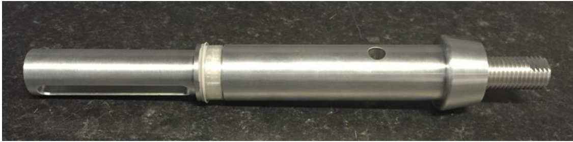
Figure 3-15: The internal element before the remainder of the muscle is constructed around it.
