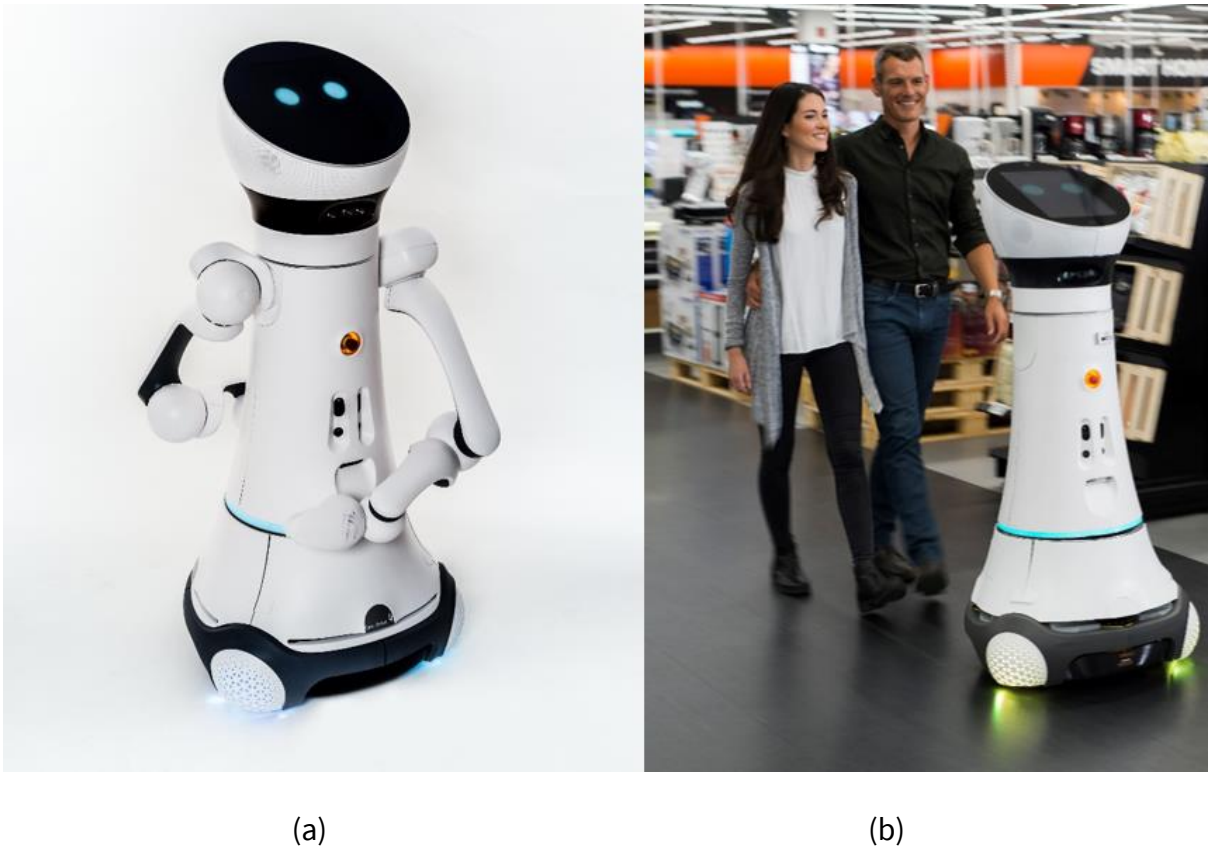
Figure 2-1: Care-o-bot 4 configured with torso, head and arms [27](a) and operating in Saturn-Markt [28] (b).
