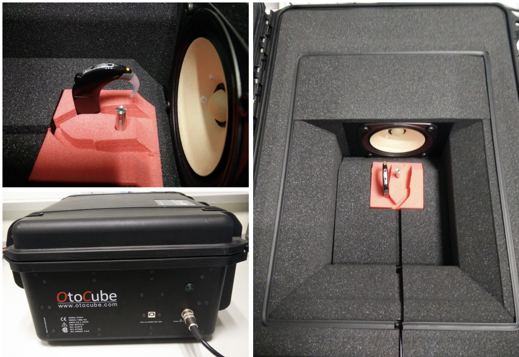
Figure 4.1: Placement of a cochlear implant (CI) in an Otocube® (Otoconsult NV, Belgium).
