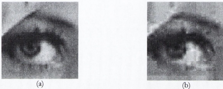
Fig. 3.10 Example of blocking effects in transform coding. Original (a) and reconstructed image (b), enlarged for clarity.
