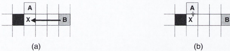
Fig. 5.38 Illustration of estimating a pixel X from a sample point B and a pixel from a neighbouring block. B is known and therefore has confidence factor of 1, while A is predicted and thus will have a lower confidence factor. A is closer to X than B however, which will “boost” its contribution to the estimate of X .
