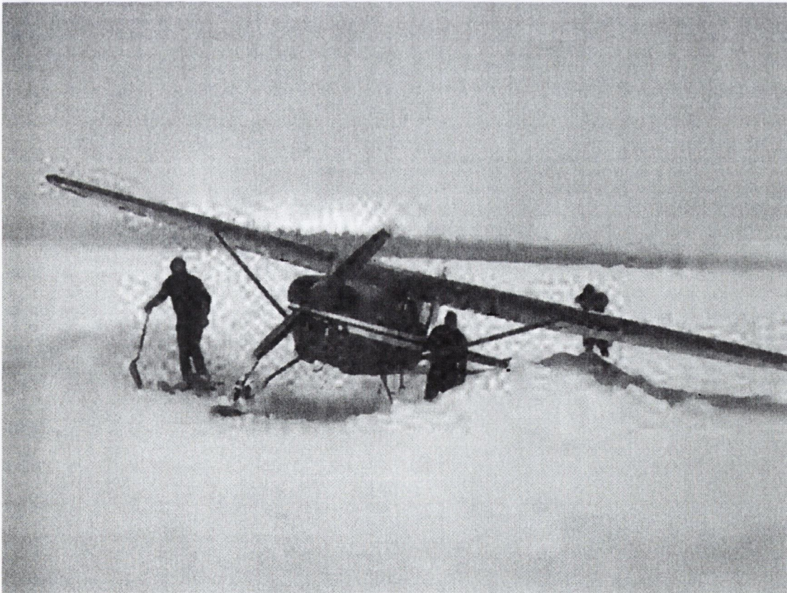
Fig. 6.15 Reconstructed Plane image at a compression ratio of 85:1 without filtering of the smooth component prior to insertion in the sample grid. The smooth image corresponds to a JPEG Q factor of 55. Subsampling factor = 4.
