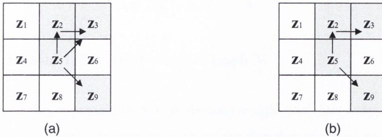
Fig. C.2 Ambiguity of 8-connectivity, addressed by m-connectivity . In (a), under 8-connectivity, z_5 may be linked to z_3 by two different “routes” which causes problems when tracing contours. Under m-connectivity , the diagonal link from z_5 to z_3 is not allowed because these pixels connect to each other through 4-connectivity.
