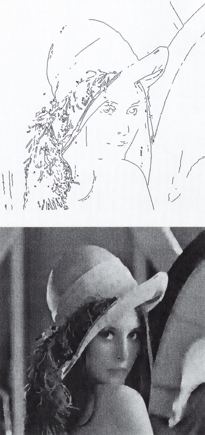
Fig. 6.2 Contour-map and reconstructed image for 512x512 “Lena” image, using a subsampling factor of 8, no smooth component compression, no texture, and the Sobel edge operator, and a contour bit-rate of 0.0514 bpp.
