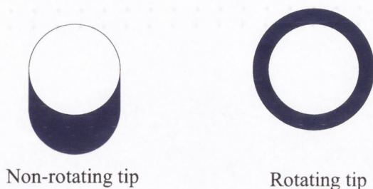
Figure 2.14: This figure shows how the metal would be evaporated onto a fibre when it is static or rotating.
