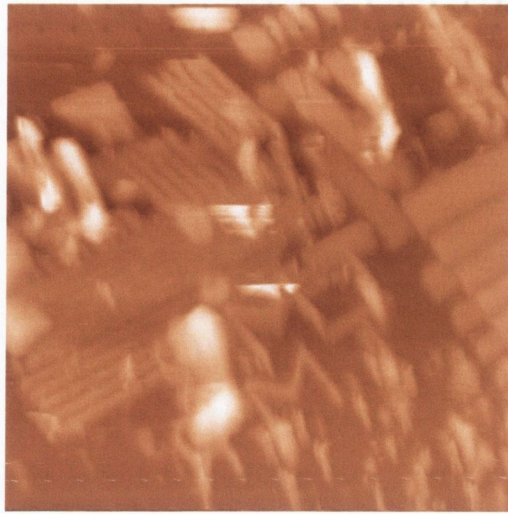
Figure 3.14: This scan shows a shear-force scan of one of the test samples used. A double-tip effect occurred in this scan. The two sensing elements of the tip have a distance of approximately 1.4 \mu\text{m} .
