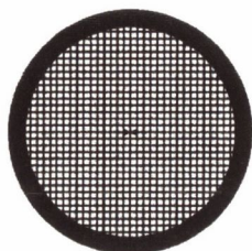
Figure 3.13 TEM grid, diameter 3mm
