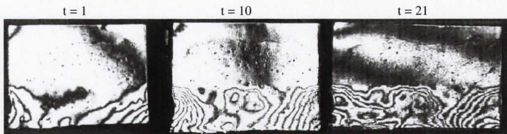
Figure 5: Horizontal component interferograms for three different times after grating application for specimen (ii), the composite beam. Time is in days
