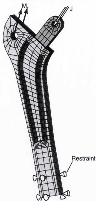
Figure 3.17. Mesh of experimental model used to study damage accumulation under conditions closer to a real femoral replacement. Selected nodal restraints are included to illustrate the boundary conditions for the model.
