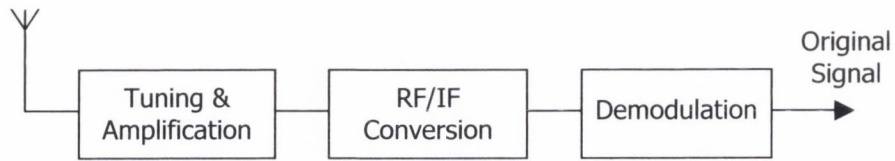
Figure 1.1 – Typical Receiver Using Traditional Analogue Hardware
