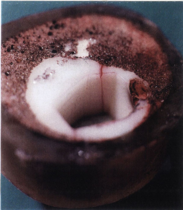
Figure F5: Photographs of the Müller inner cement mantles. The samples have been cyclically loaded, sectioned and push out tests have been performed. Damage along the cement/prosthesis interface is evident.
