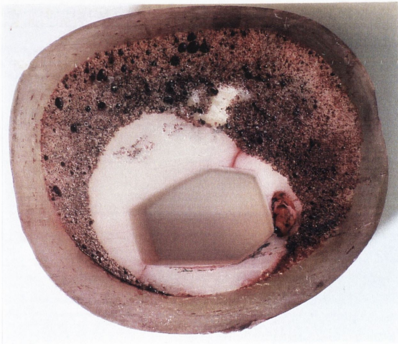
Figure F2: Photographs of the Müller cement mantles. The samples have been cyclically loaded, sectioned and push out tests have been performed. Damage in the cement mantle and along the interfaces is apparent.
