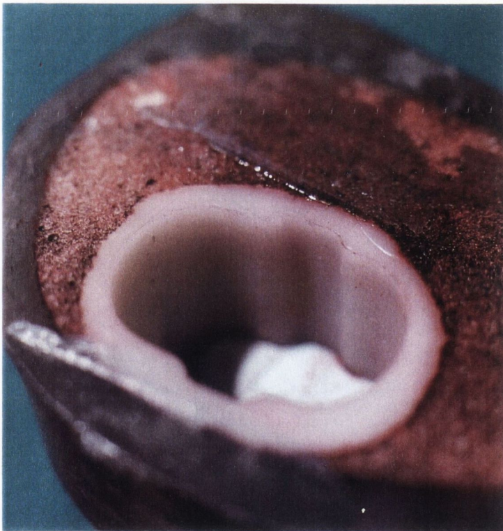
Figure F4: Photographs of the Lubinus inner cement mantles. The samples have been cyclically loaded, sectioned and push out tests have been performed. Damage along the cement/prosthesis interface is evident.
