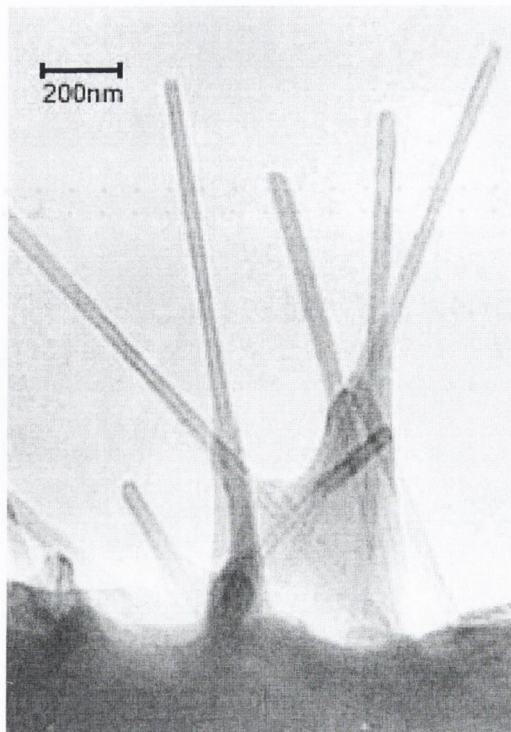
Figure 3.8 TEM of Arc Discharge Method MWNT Composite.
