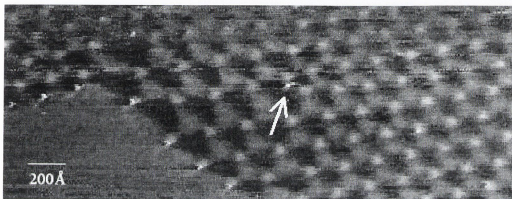
Figure 7.4 An edge dislocation in the PmPV film.
