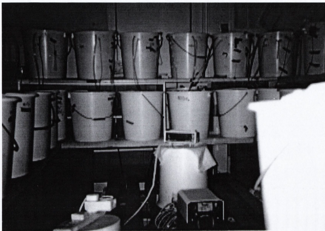
Fig. 4.3: Photograph of the experimental setup, showing microcosm units (vessels- higher tier and reservoirs -lower tier) and 24 channel peristaltic pump
