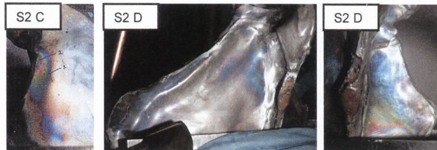
Figure 4.2 Photoelastic stress analysis plots for scapula 2 at a 1.6 kN load, C refers to the costal view and D refers to the dorsal view.
