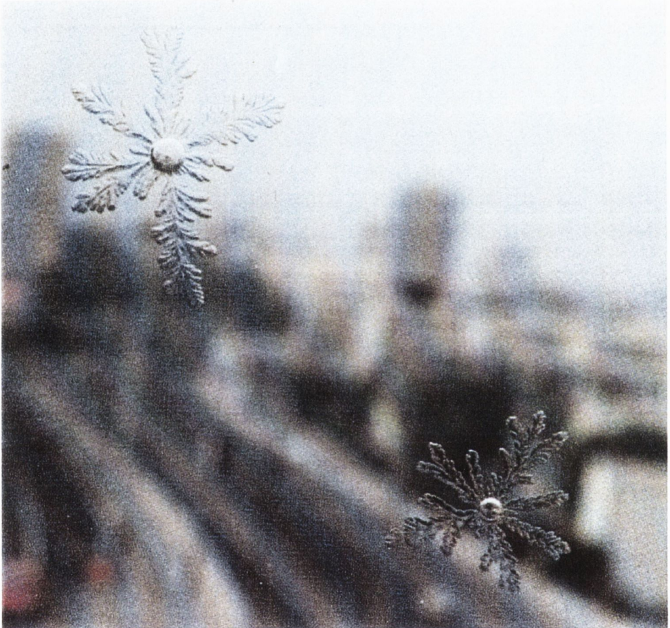
4. Spontaneous cracks in this window pane developed with a fractal structure (Guyon and Stanley, 1991).
