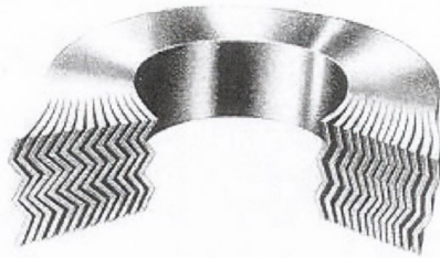
Figure 2.9: Die formed graphite ring after compression (Source: [26])
