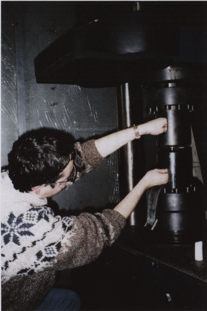
Figure 6.8: Fatigue Testing of Rolled Fasteners
