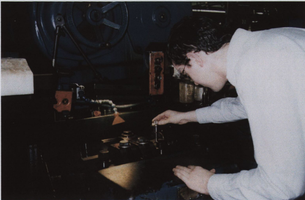
Figure 6.4: Thread Rolling of the fasteners
