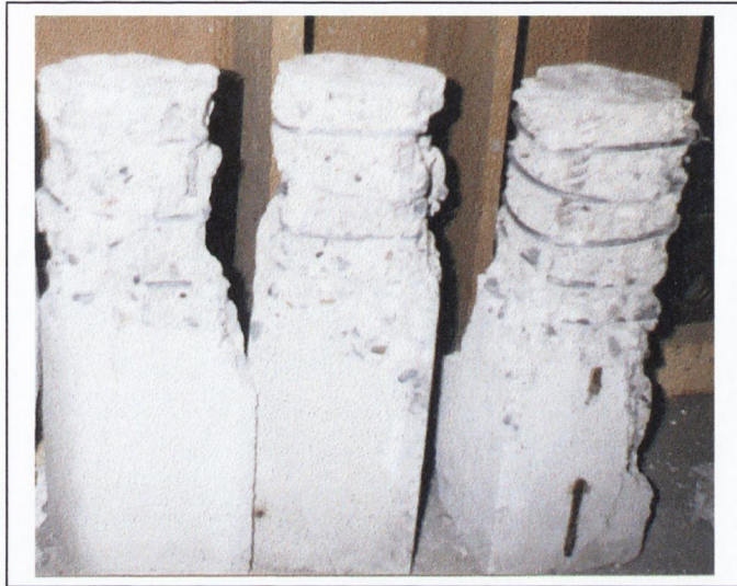
Figure 4.1: Typical failure of conventionally reinforced stub columns with and without wireballs
