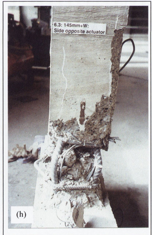
Figure 5.5: Specimens post-failure: (e) and (f): C6.4(125,W,40) and (g) and (h): C6.3(145,W,40)
