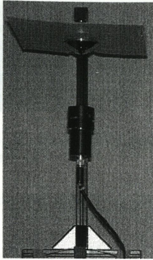
Fig. 2.13: The SVAVISCA omnidirectional camera with a specialised mirror
